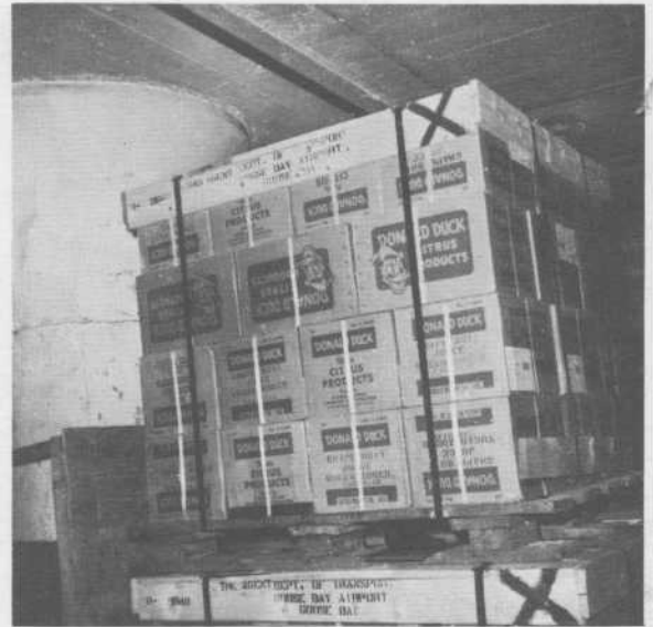
One of the collapsible box pallets suggested by Mr. Girard is loaded with fruit juice and ready to be shipped north during the annual Arctic resupply.
