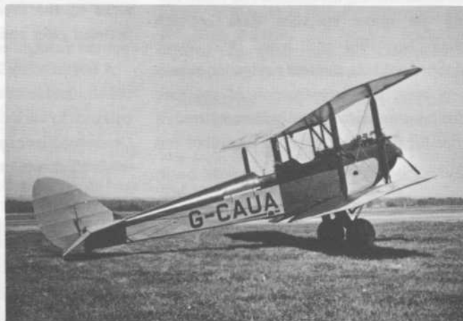
The De Havilland DH60 Cirrus Moth was the forerunner of the familiar Tiger Moth. Powered by an 85 h.p. engine, it had a top speed of 85 m.p.h., range of 430 miles and ceiling of 17,300 feet.
