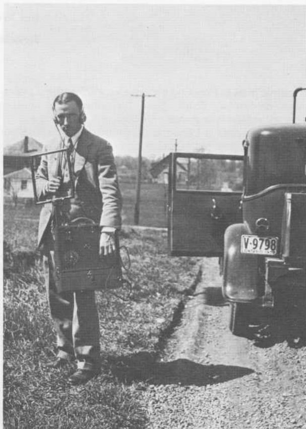
In 1930 Ralph Bunt, above, investigated radio interference with the aid of headphones, a portable receiver and loop antenna. Today John Demers (in fur hat) and Bob Coxe, Ottawa, are shown, left, tracing sources of interference by means of an all-wave communications receiver mounted in a specially-constructed radio van.
