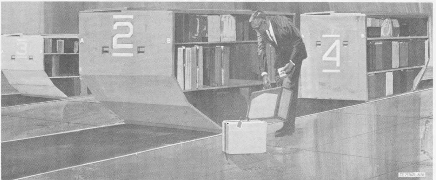
In this illustration from a Boeing brochure, it is proposed that baggage handling be facilitated by means of numbered and, perhaps, color-coded baggage containers with a relatively small number of compartments. These would go on and off the aircraft intact and be delivered by conveyor belts into the terminal where passengers could find their luggage with ease.
