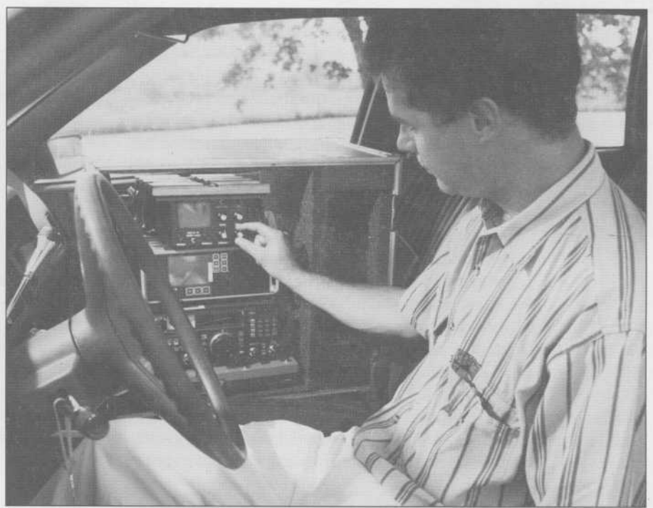
Radio Inspector Robert Régimbald adjusts the settings on the Techcomm Direction-Finding System, one of two systems the Department is evaluating, to find a signal's direction.
